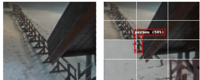
Figure 8: The full image (left) does not trigger a person detection, but tiling and combination with the background cause the fence to be interpreted as a person.
